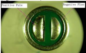
**Soldering Time:** <3 seconds total. (Iron contact to removal time). Soldering alternation between positive pole and negative pole: Less than 10 seconds.
