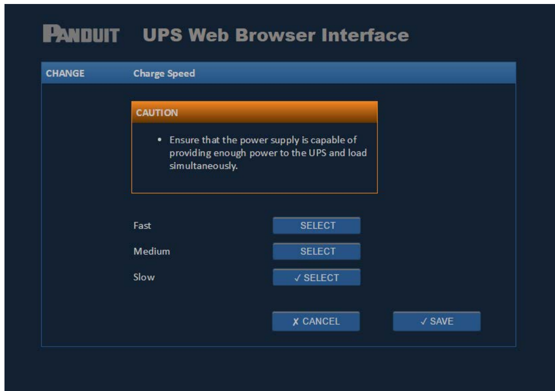
Figure 8: UPS Web Browser Interface - Charge Speed
