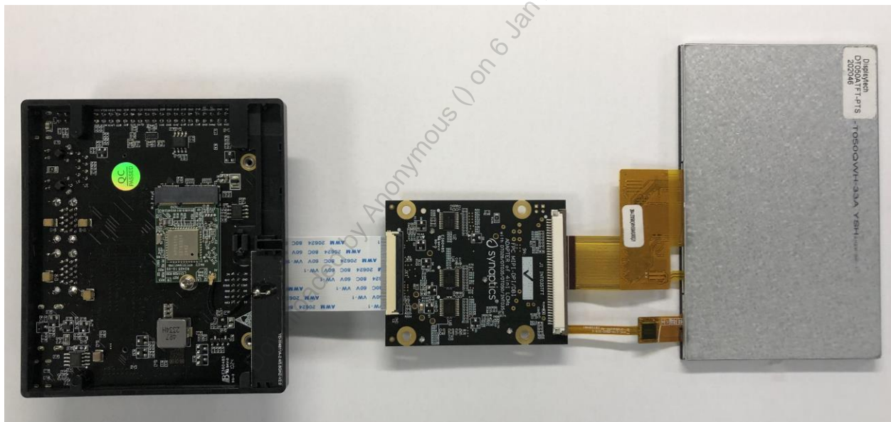
Figure 5. Complete connection to the 4-in-1 LCM Adapter Board (bottom view)
