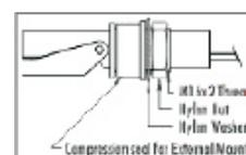
Turn the fixing nut only until the compression seal/grommet starts to deform.
