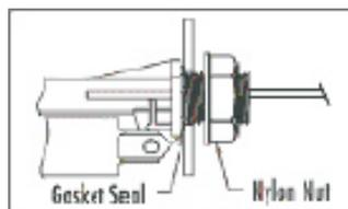
Hold the float switch firmly, ensuring that the orientation of the float is correct and that the sealing washer/gasket is not impaired, and tighten the nut, until finger tight.
