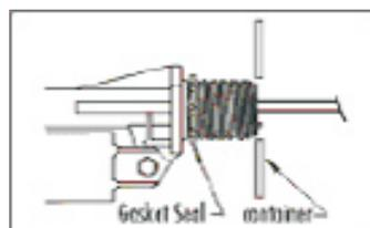
Feed the fixing nut over the connecting lead/s and position on the float switch thread, ready for tightening.
