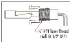
Apply a compatible thread sealing compound, or tape, to the thread and engage the assembly in the threaded tank wall. Rotate the assembly until it is finger tight in the thread.
