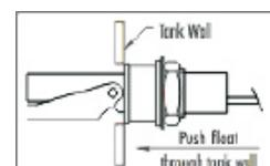
Hold the float assembly by the cable entry end, using the flats provided, and carefully tighten the fixing nut to a maximum torque of 2.0 lb ft (2.67Nm).
