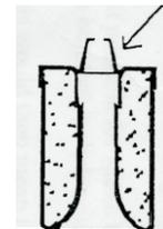
Fit the locking cone on the cable, feed the cable through the counterweight and insert it into the base of the counterweight to lock the counterweight in the required position.
