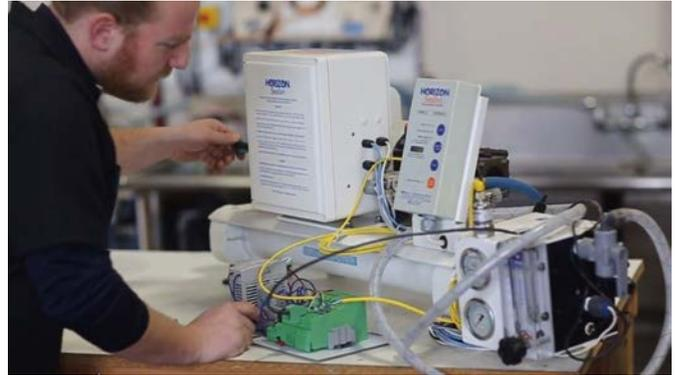
S3 Maritime uses Phoenix Contact's ILC controllers to program and communicate via PROFINET and Modbus.
